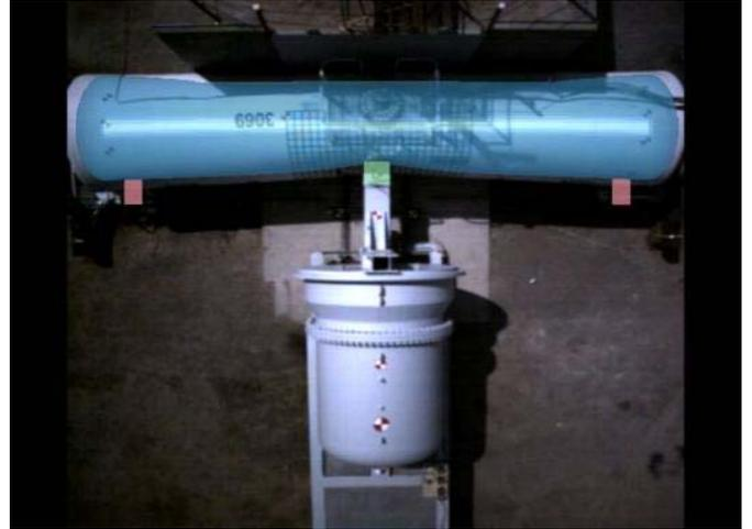
**Figure 6. Overlay of Deformed Shape from FEA Simulation on Still Frame from High-Speed Movie**
