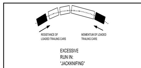
Typically, the rail car does not turn over (initially) but a wheel climbs over the rail or a rail turns over and eliminates the ability of the track structure to contain the train. Jackknifing is often exacerbated by combinations of long and short cars coupled together.
