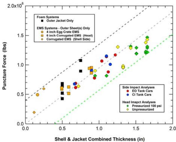
Figure 6. EMS puncture forces as a function of outer layer thickness.
