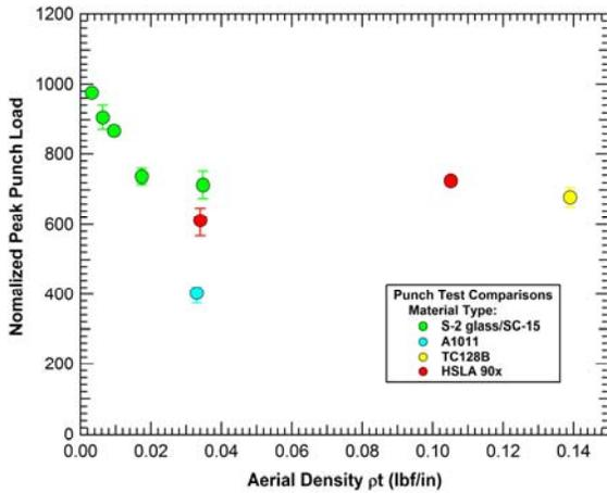
Figure 7. Normalized peak punch test loads versus aerial density for various materials.
