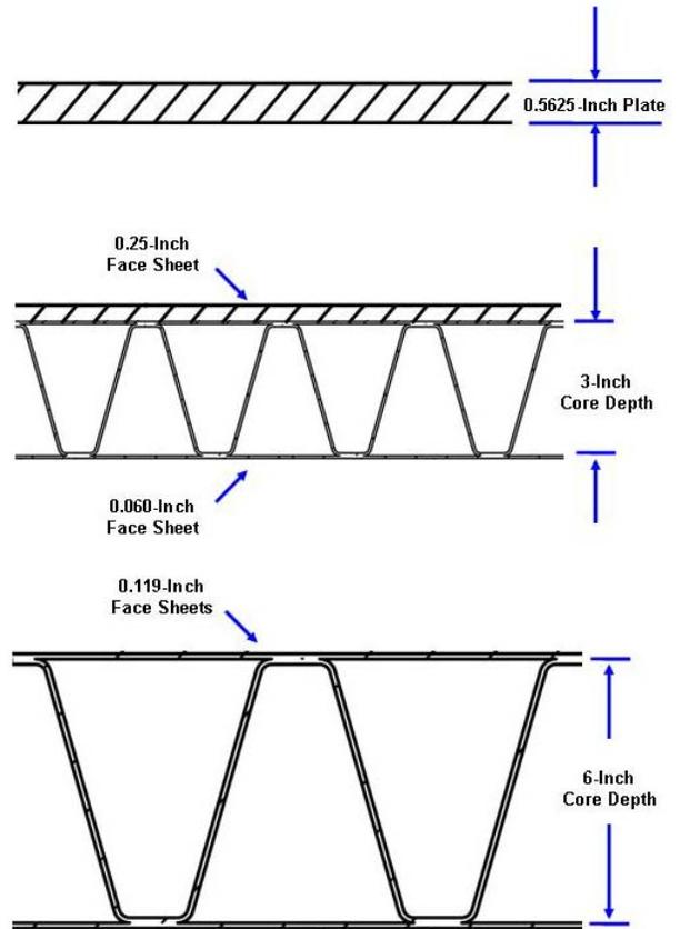
Figure 4. Alternative EMS tank protection concepts.
