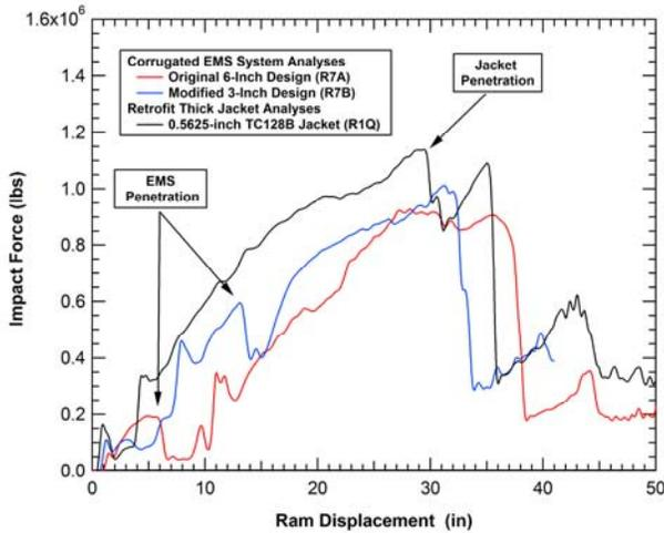
Figure 5. Comparison of the force-deflection behaviors for the Corrugated EMS concepts.
