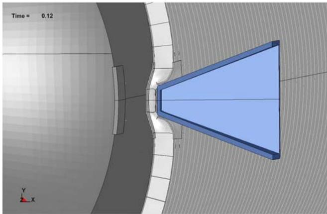
Figure 3. Calculated intermediate impact damage for a 4-inch egg crate EMS system.
