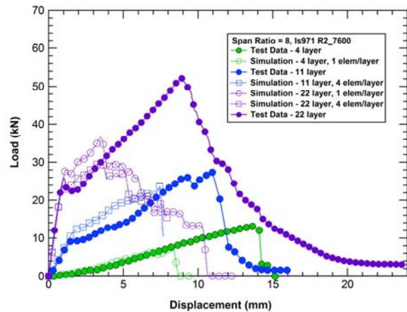
Figure 8. Comparison of punch test data and simulations.
