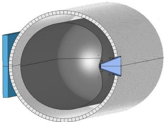
Figure 2. Calculated side impact response and penetration for a 4-inch egg crate EMS system.
