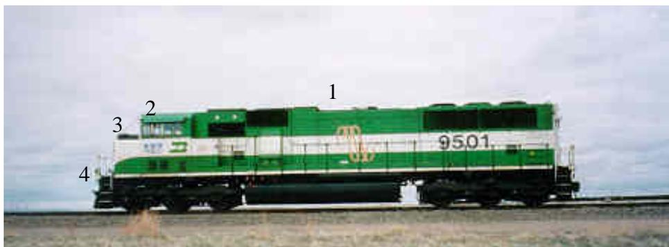
**Figure 1. Horn Installation Locations**
