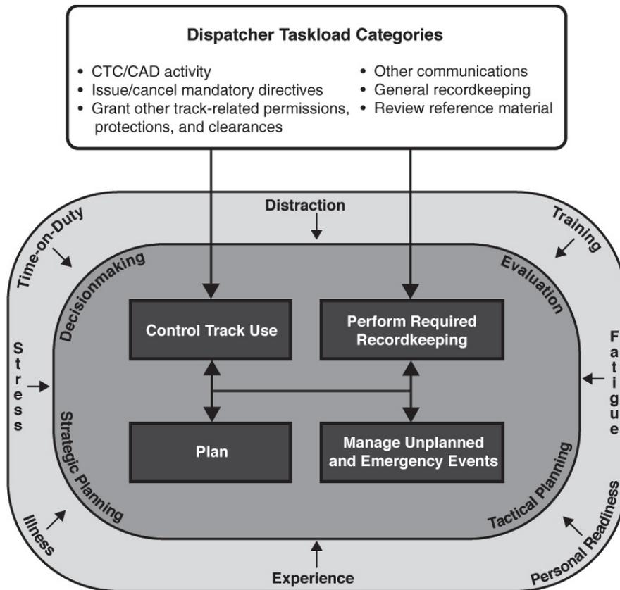
Figure 3. A preliminary model of railroad dispatching
