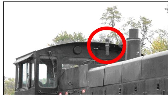
Figure 4. GPS Tracking System
