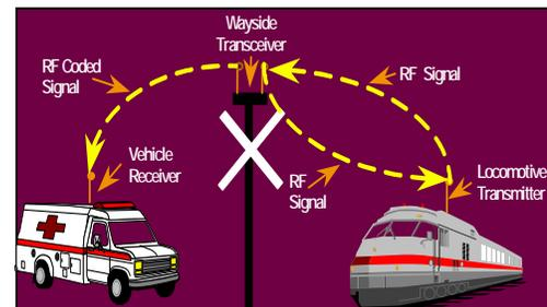
Figure 3. Three-point VPAS Concept
