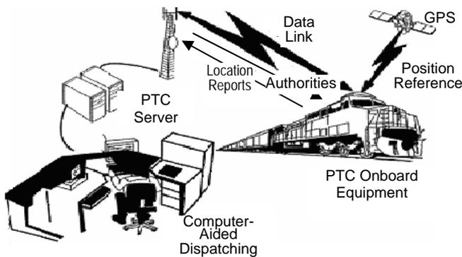
Figure 1. PTC System Flow
