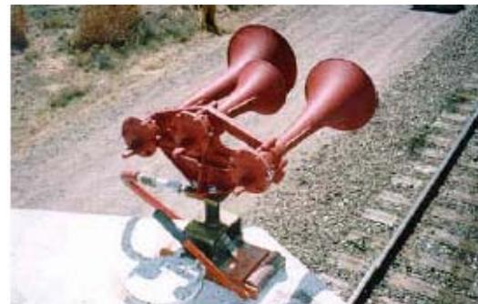
**Figure 4. Three-Chime Train Horn Tested in Mundelein**
