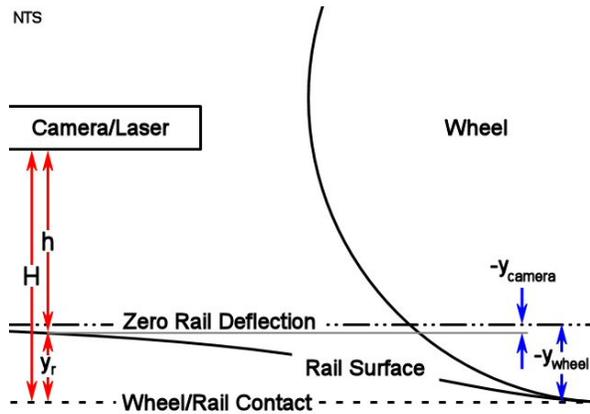
Figure 2. Rail Deflection/Sensor Measurement
