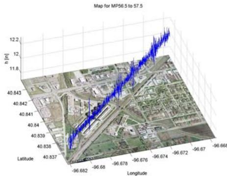
Figure 5. Relative displacement vs. location
