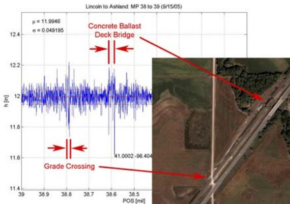
Figure 6. Displacement vs. location
