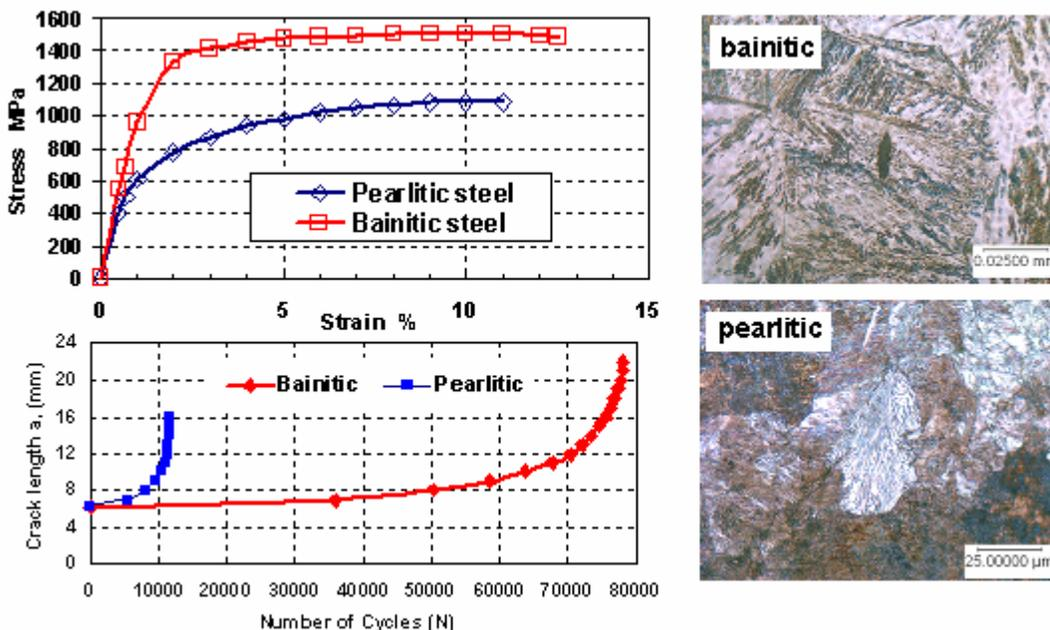
**Figure 1. Microstructure - Mechanical properties and fatigue relationships of Bainitic and pearlitic rail steels.**
