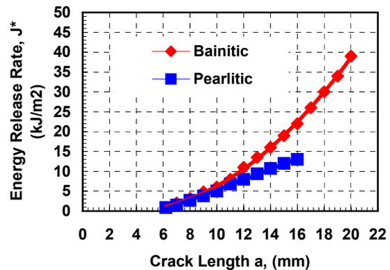
**Figure 2: Energy release rate, J\*, versus the fatigue crack length, a.**
