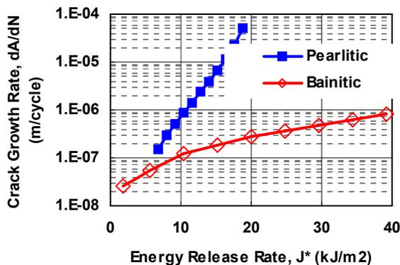
Figure 3 Crack growth rate,  $da/dN$ , versus energy release rate,  $J^*$ .
