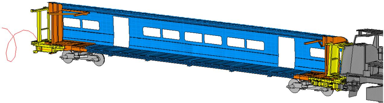
**Figure 1. Detailed Nonlinear FEA Model for Analysis of Colliding Trains**
