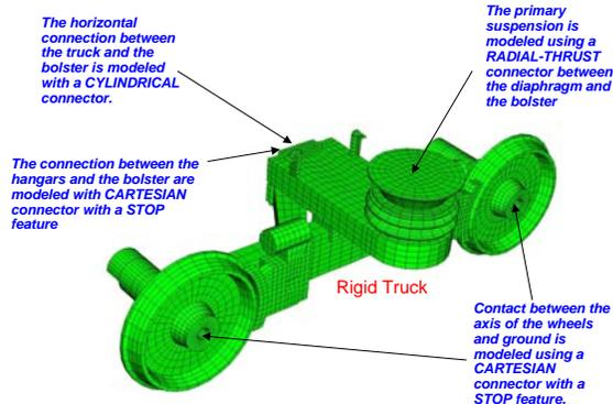
Figure 5. Cab Car Truck Portion of Model
