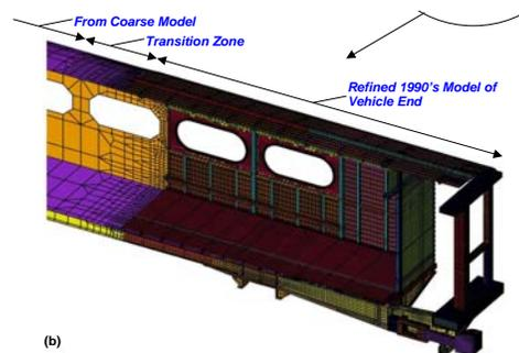
**Figure 3. Cab Car Portion of Model**
