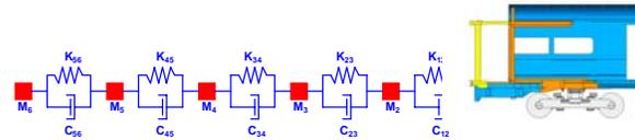
Figure 6. Trailing Equipment Portion of Model
