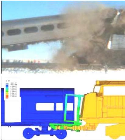
**Figure 8. Conventional Train-to-Train Test Result and CEM Train-to-Train Test Prediction**
