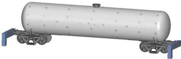
Figure 4. Updated model of a 105J500W pressure tank car.
