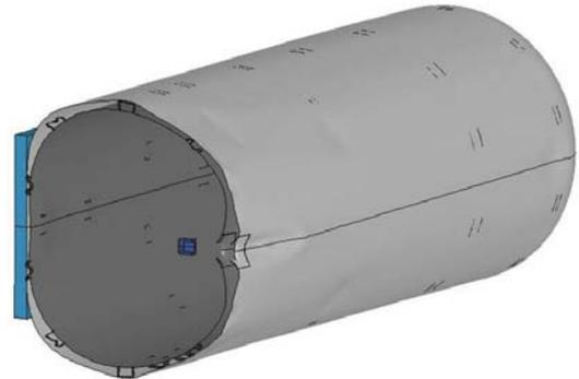
Figure 12. Simplified tank model analysis with Bao-Wierzbicki failure assessment.
