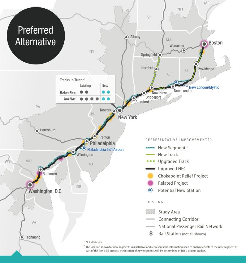
The Preferred Alternative includes improvements to bring the NEC to a state of good repair and relieve chokepoints that cause delay. It adds new track to grow the NEC to four tracks at most locations, with more tracks in areas with the greatest demand. In addition, the Preferred Alternative integrates direct service on the Hartford/Springfield Line into the NEC, with upgraded track and electrification.
