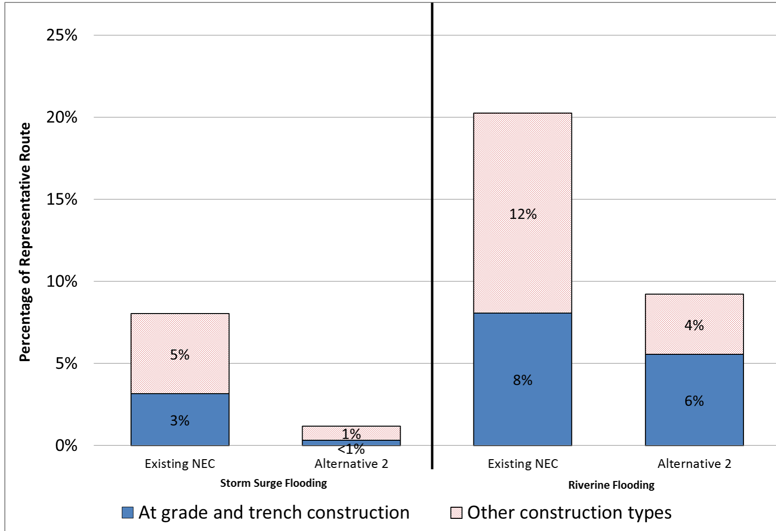
Figure 7.15-12: Current Climate Conditions (Storm Surge and Riverine Flooding): New Haven-Hartford-Providence – Construction Type – Total Percentage of Representative Route of Alternative 2 and the Existing NEC at Risk
