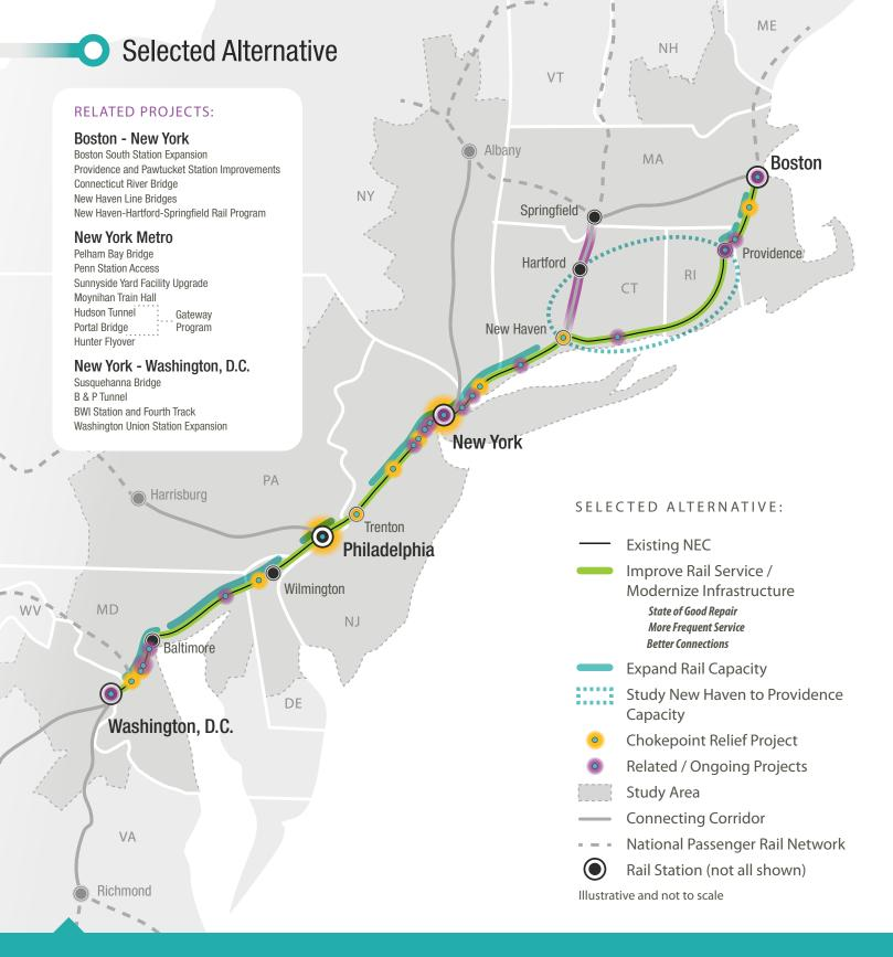
Grows the NEC to a 4-6 track modernized, integrated rail network with sufficient capacity to accommodate a significant increase in intercity and commuter rail service, greatly improve reliability, and reduce travel time.
