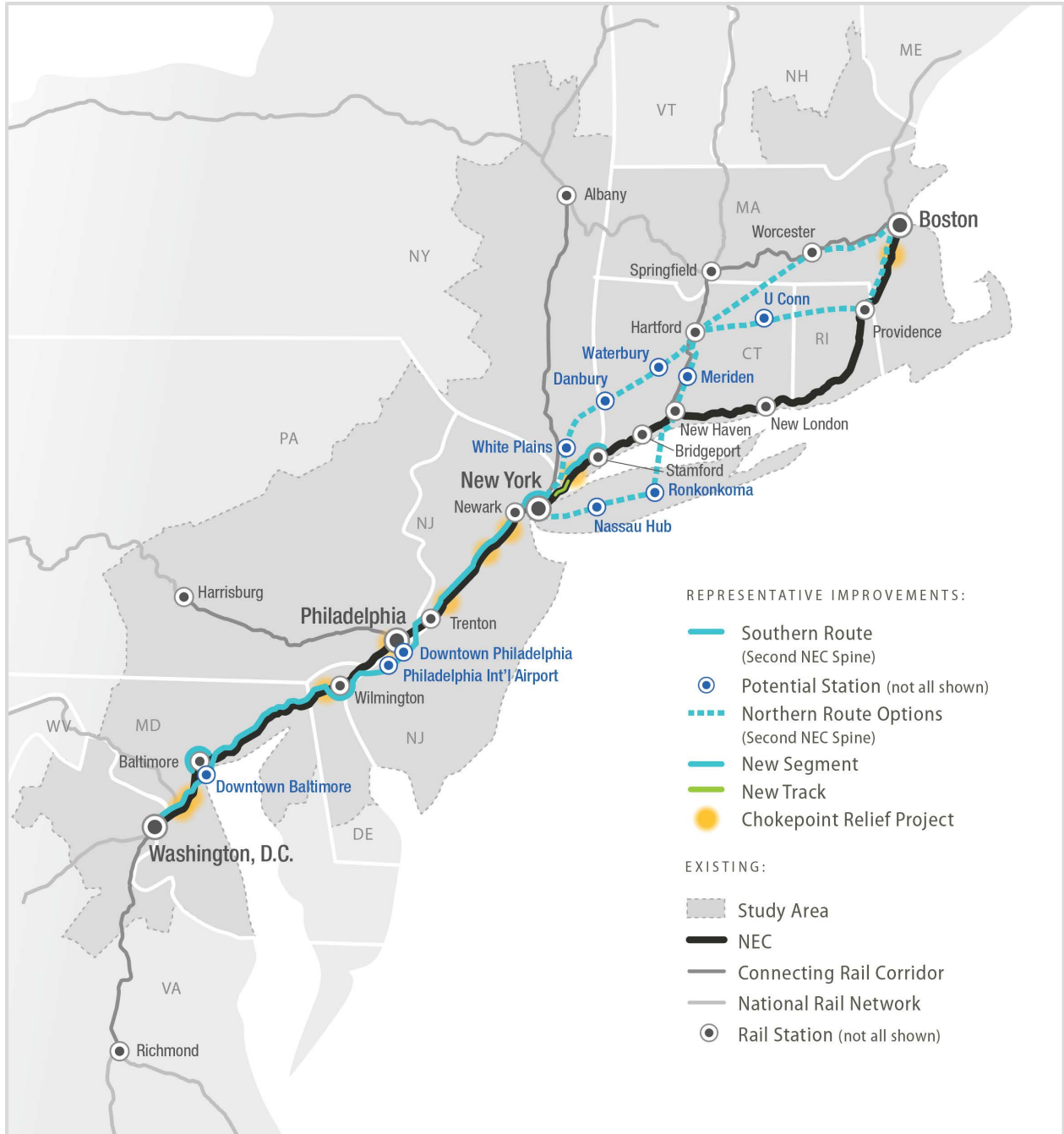
Figure 4-6: Alternative 3 (Chokepoint, New Track, and New Segment Locations)
